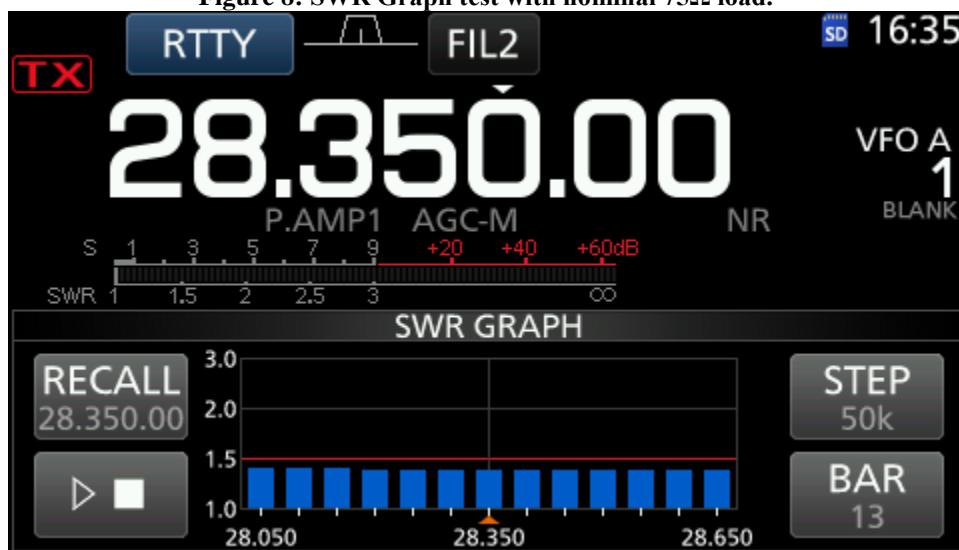
Figure 8: SWR Graph test with nominal 75Ω load.
