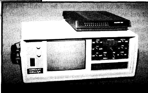
Camera tilt and zoom are remotely controlled from the portable receiver/display unit.
