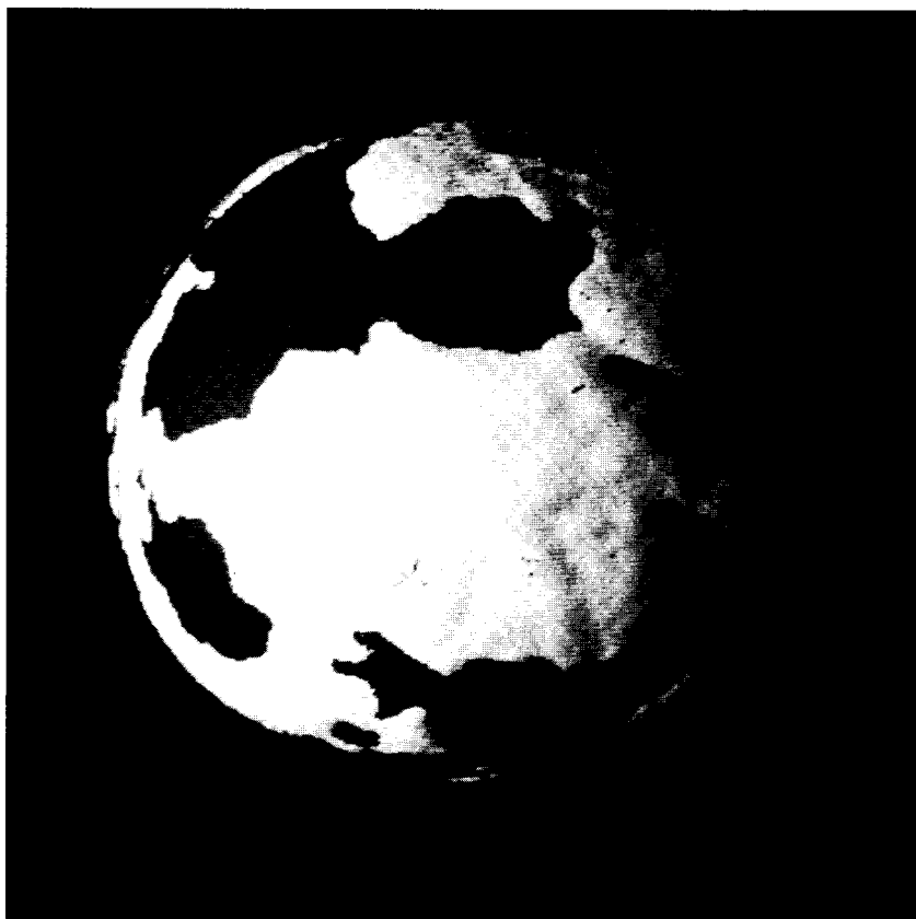
Photo 3—An fBM image mapped onto a sphere and shaded according to Eqn. 16. The position of the source was chosen 35 degrees offset from the observer and the illumination values were banded and normalized over a range of 0-255 with the seas (for r = rsph ) ranging from 1 to 127 and the land masses from 128 to 255.
