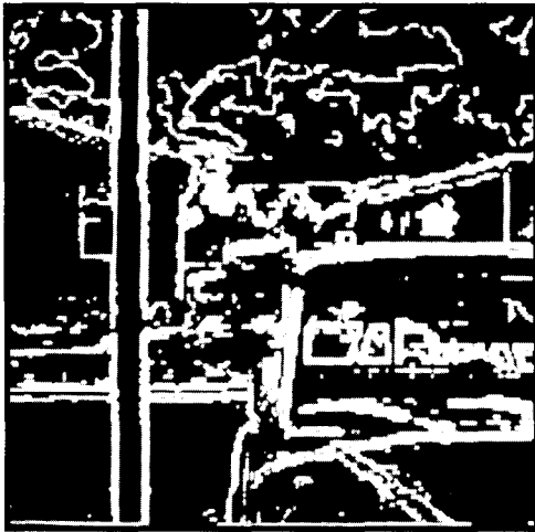
Figure 7—The Robert's edge enhancement of Figure 2 with every pixel > 15 set to 255 and all pixels ≤ 15 set to 0.
