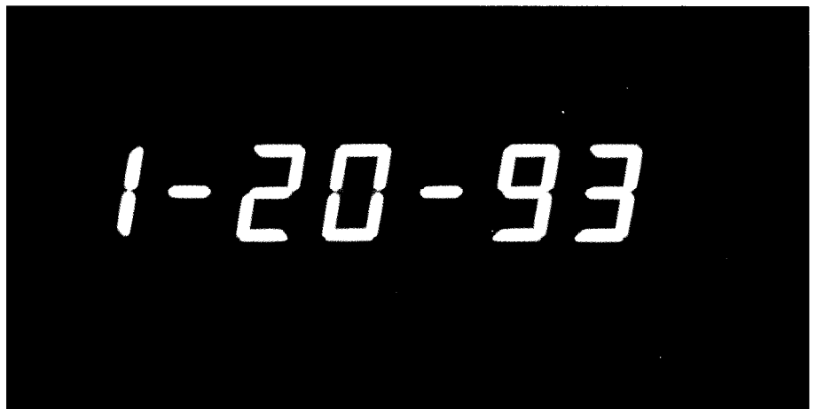
Photo 1-The MAX7219 makes the once-cumbersome job of driving a row of seven-segment LED displays a piece of cake.
