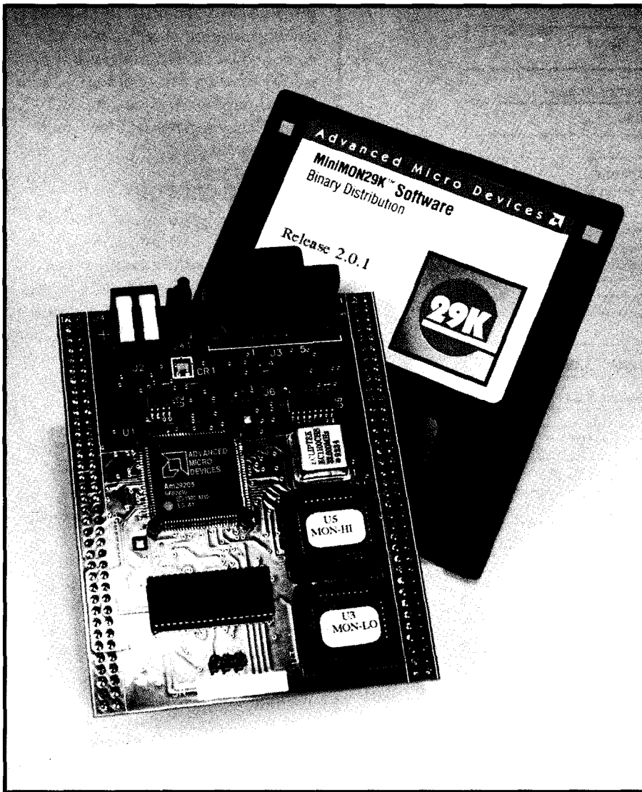
Photo I--The tiny SA-29205 demo board available from AMD allows the engineer to test drive the AM29205 embedded RISC processor without spending time trying to get the hardware working.
