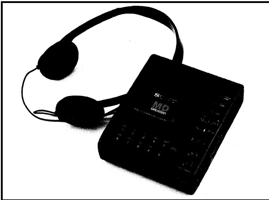
Photo 1—About the size of first-generation portable CD players, the portable MD unit allows both playback and recording in a compact package. A 1-megabit memory chip built into the playback section eliminates skipping due to shocks or bumps.
