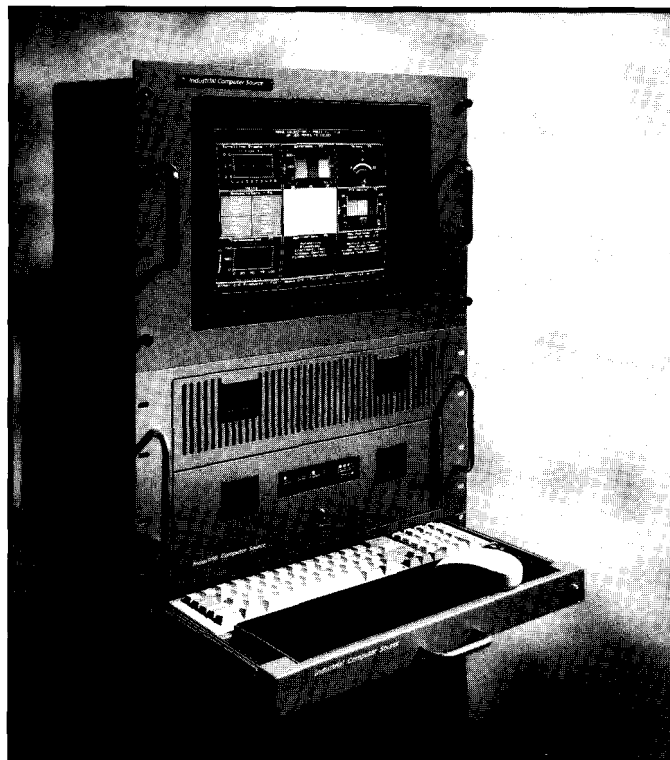
Photo 1—The Industrial Computer Source 6200-UMR rack-mount packaging system.
