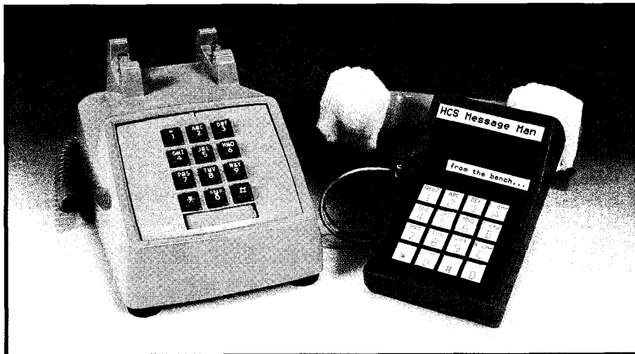
Photo 1—The Message Man interfaces with the telephone through the handset. A microphone and speaker are held onto the handset with strips of Velcro. The self-contained unit displays messages on a single-line 16-character LCD display while it accepts user input on a 16-button keypad.
