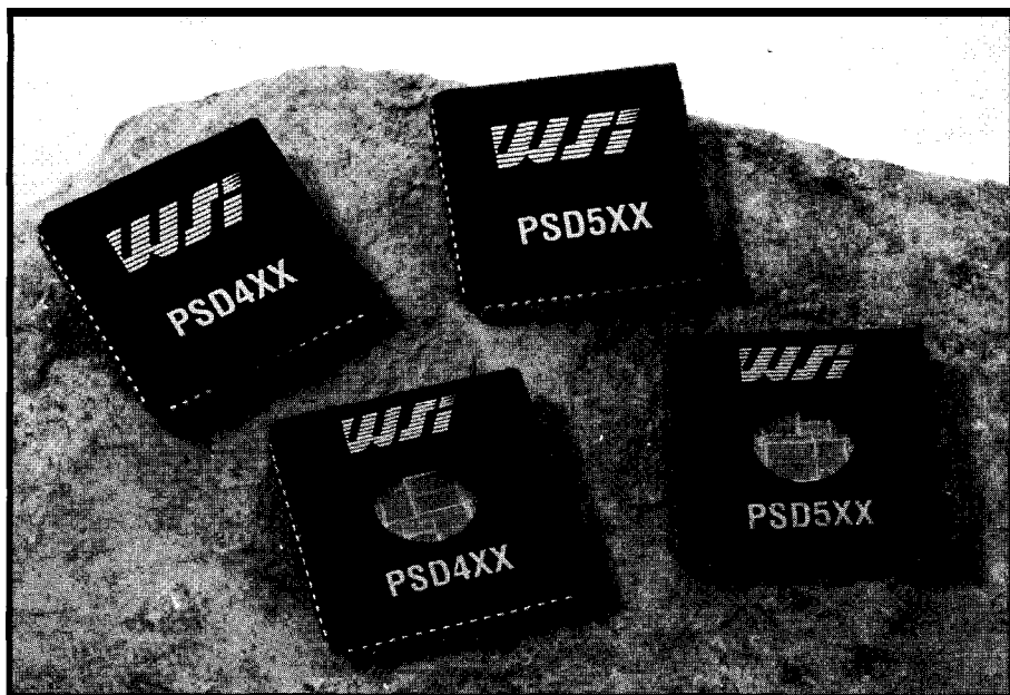
Photo 1—Although the new PSD4xx and PSD5xx series of chips from WSI present the same amount of memory, EPROM access times have left their predecessors far behind. An additional 5 bits to Port C and two 8-bit ports—D and E—have made these chips into a more powerful 68-pin general-purpose PLD.
