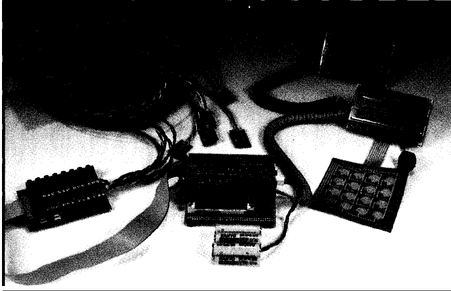
Photo 3—The complete system includes processor board, interfaces, displays, keypad, sensors, and battery power management.
