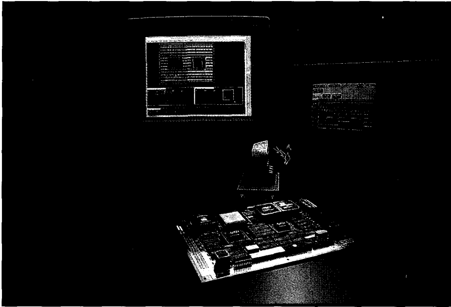
Photo 2—The Aptix AXB-GP2 general-purpose FPCB (Field Programmable Circuit Board) contains over 1700 through-holes laid out in an area of 100×100×300 mils and allows programmable control of the actual PC board layout.
