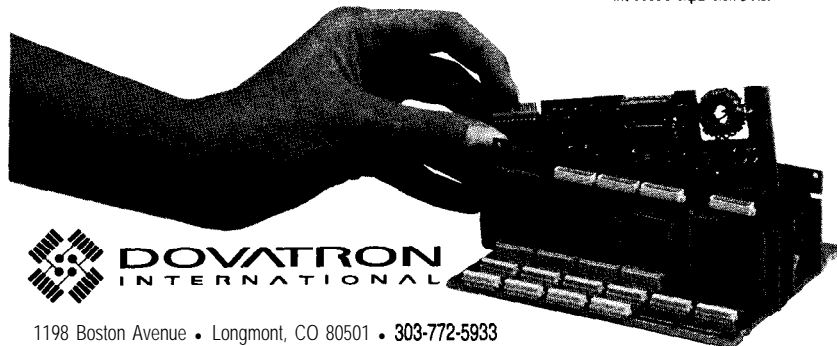
8680 XT Kit Measures 5.3" x 4.1" x 1" Includes 2 expansion slots.
