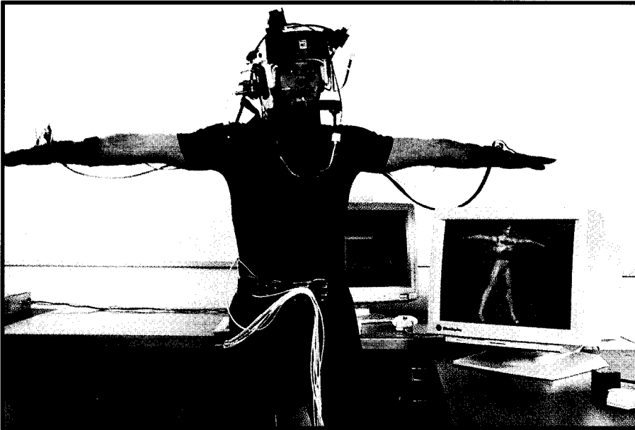
Photo 2-The SimGraphics VActor setup uses input sensory devices connected to a human host in order to animate computer-generated characters.
