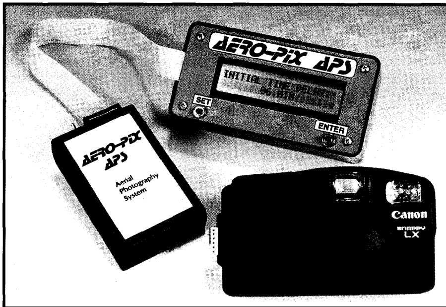
Photo 1--The Aero-Pix APS consists of three elements: the main controller (bottom left), the programming interface (top center), and, of course, the camera. The programming interface is removed from the main controller before sending the controller and the camera a/oft.
