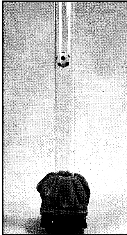
Photo 1—The PID-Pong Challenge is to come up with a scheme that will automatically maintain the pin-pong ball in one position in a tube on a cushion of air.
