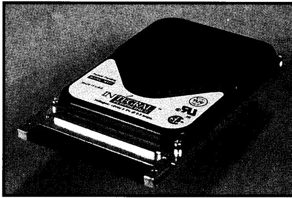
Photo 1—A Type III PCMCIA card typically houses the rotating media of a hard drive.
