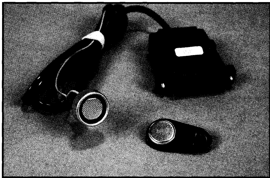
Photo 3—Dallas Semiconductor can supply a wide variety of touch probes and sockets which easily interface to either a serial or parallel port on a PC.
