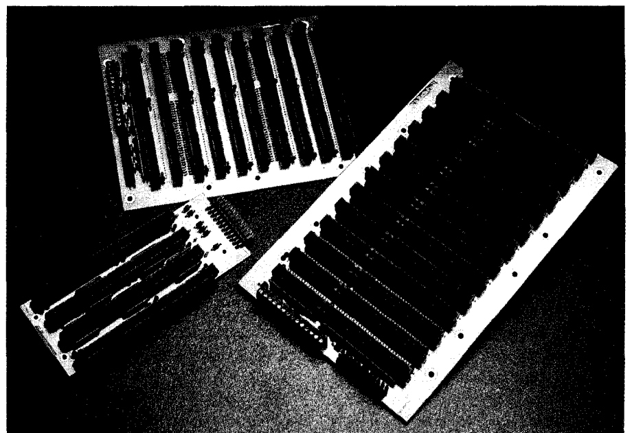
Photo 2: Conventional ISA/AT passive backplanes such as those from Microbus provide economical system solutions in a variety of sizes.
