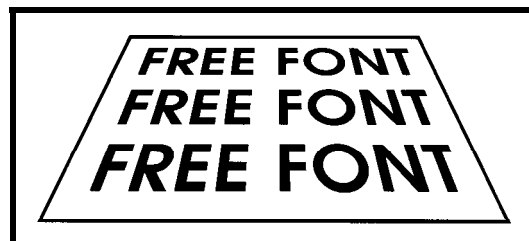
Figure 2—The Star-wars nonlinear graphics transform gives the effect shown here. Jo create if, select a tilt angle \theta where 0^\circ is flat and 90^\circ is vertical. Predefine a tilt factor with geometric constant k , k = \text{fullheight fan } \theta . The nonlinear transform is then x' = xk/(k+y) , y' = yk/(k+y) .
