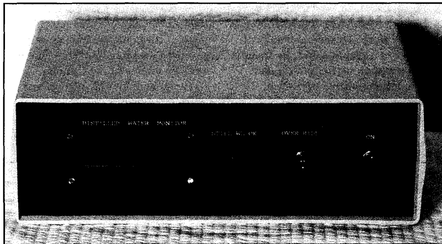
Photo 2—The display unit can be conveniently located where it is easy to monitor. It connects to the oscillator head via a 3-wire cable.
