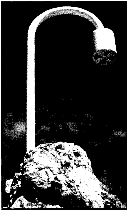
Photo 1-A field mill measures the static and slowly changing components of electric fields associated with a thunderstorm.
