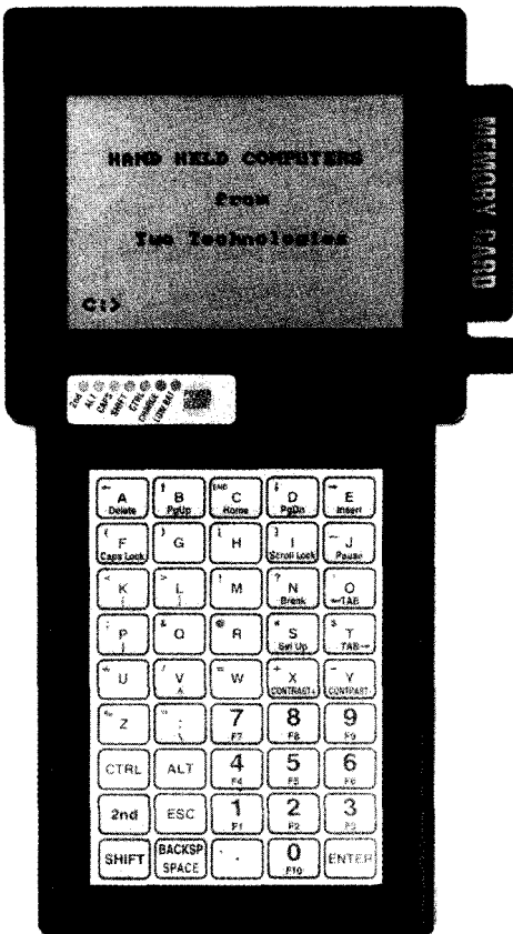
Photo 8: Operating from batteries or a wall pack, hand-held PCs like this PC-Lite unit from Two Technologies permit the embedded PC to travel anywhere for on-site data entry and collection, machine setup, data acquisition, and other remote computing needs.
