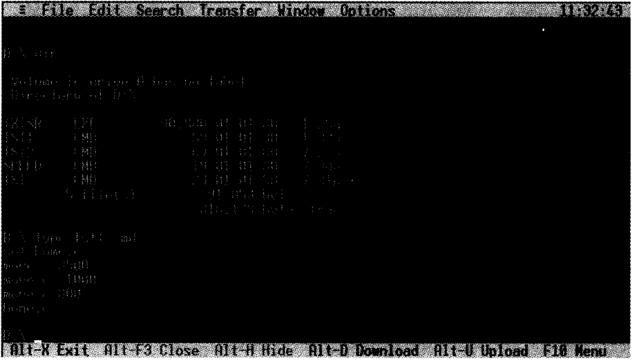
Photo 8: The Indexer LPT executable resides on virtual drive D along with the .CMD application file. The DOS TYPE command reveals the contents of TST1 . CMD .
