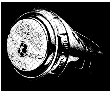
Photo 2—Talk about keeping your data close at hand! The decoder ring actually has a touch memory device mounted on it. Touching the ring to any reader instantly identifies the wearer.
