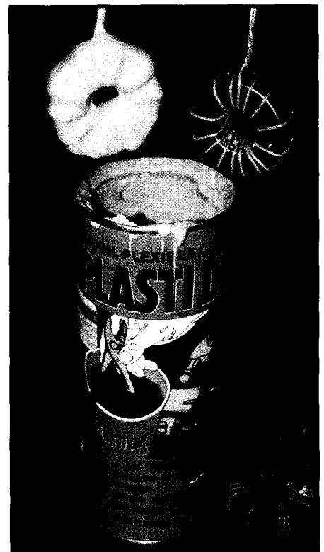
Photo 1—Because the ferrite is conductive, I coated the toroid assembly using a plastic dip process, completely covering each unit.
