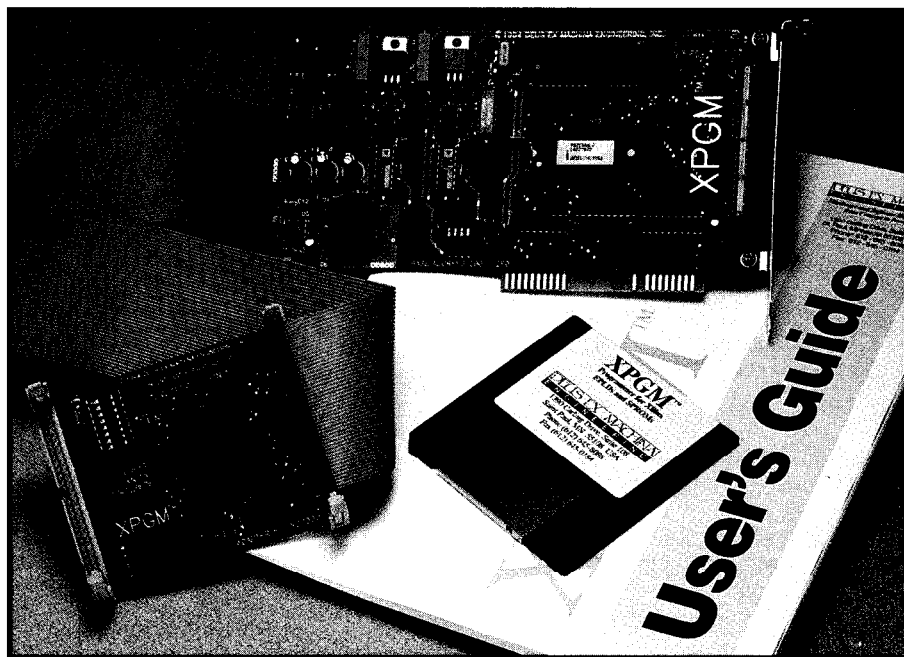
Photo 1—XPGM is a Xilinx-certified programmer manufactured by DeusEx Machina Engineering and distributed by Digi-Key.
