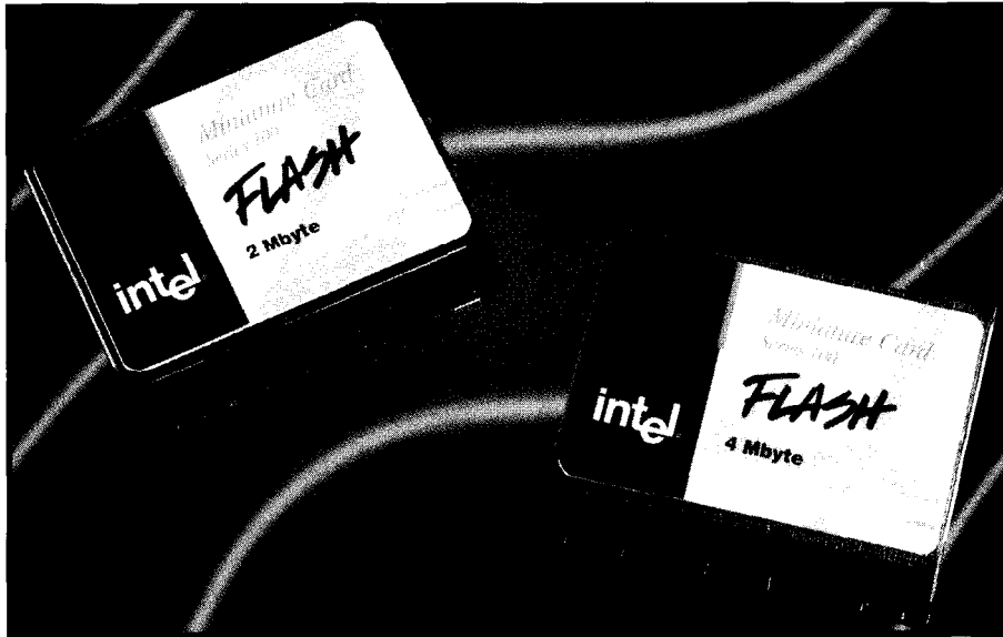
Photo 2—The MC is effectively a big memory chip that accommodates SRAM and DRAM as well as flash.
