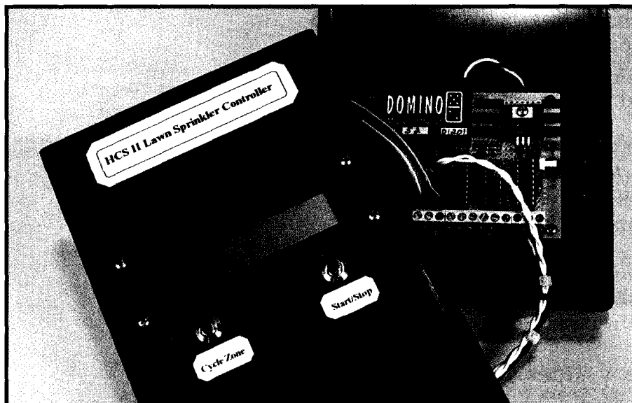
Photo 3--Here's the complete lawn-sprinkler controller.
