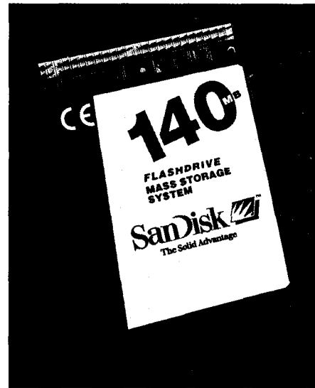
Photo 2: SanDisk's FlashDrive looks and acts like a miniature (1.8") IDE hard disk, so it's easy to use. Note the IDE interface—a high-density, 2-mm, 44-pin connector.
