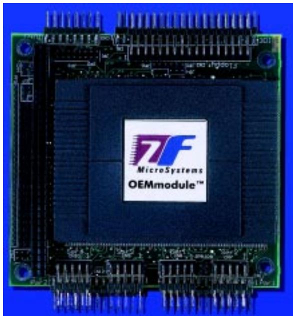
Photo 1—This PC/104 module, using ZF MicroSystems' PC/AT on a chip, contains everything we need: a 40-MHz '386 CPU, 2 MB of RAM, serial/parallel and disk I/O, BIOS, and a 512-KB SSD in a single module. At less than 2 W, this module is perfect for portable applications, like a robot.
