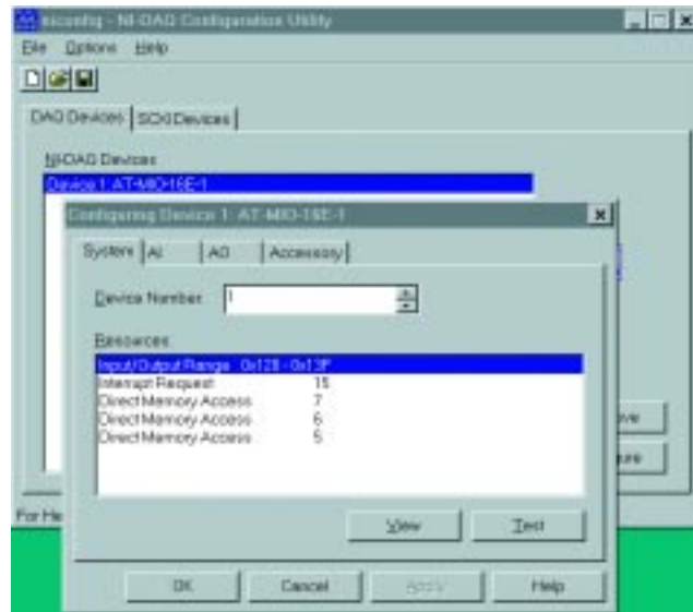
Photo 1—This is more like it. Notice that three DMA channels are used by the DAQ card.
