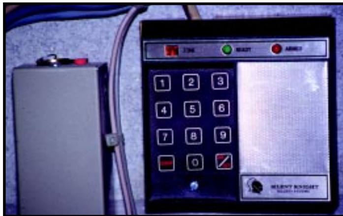
Photo 1—The alarm system PIN is entered via a keypad. The ASDL system monitors and records the time and date of all key presses.
