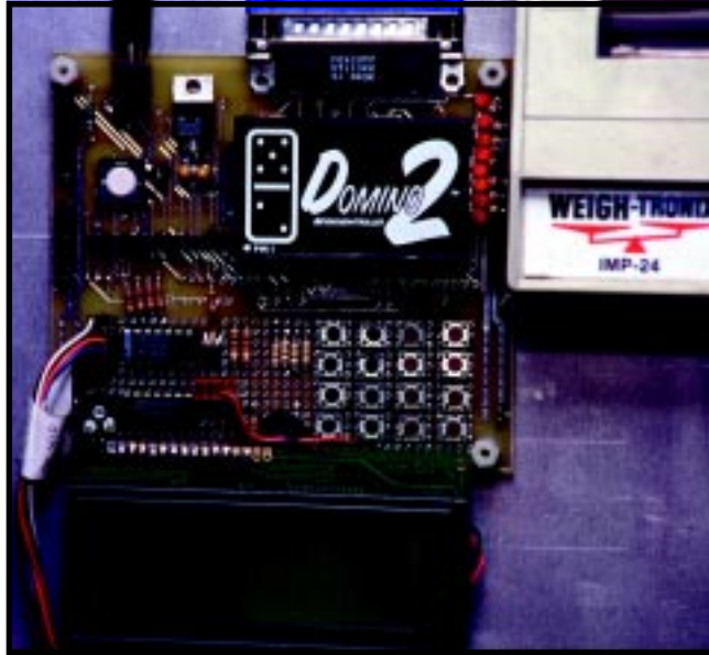
Photo 2 —The prototype ASDL system is physically assembled using a Domino development board with an LCD and keypad attached.
