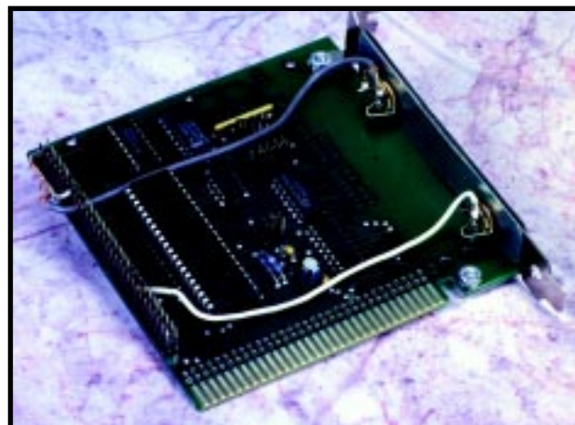
Photo 1—On this modified Prairie Digital Model 30 ADC board, the white wire is the clear (charge dump) signal and the shielded wire is for the pulse input. Note the two 1/8" phone jacks.
