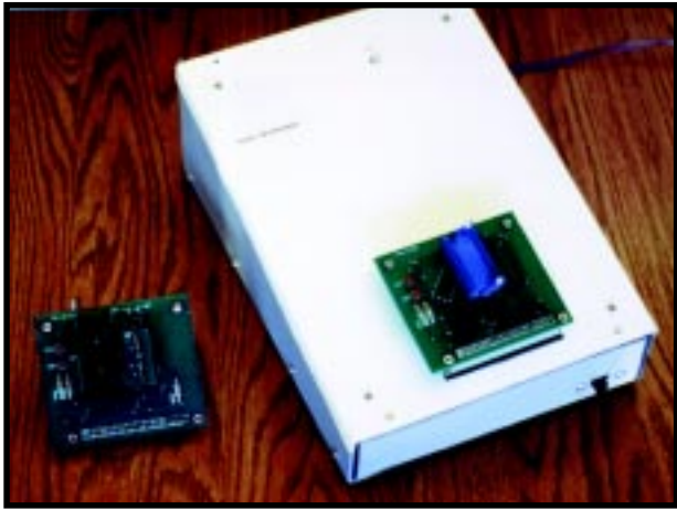
Photo 1 —Here's the completed programmer with the EPROM module installed and the PIC module beside it. There are no buttons or knobs. The entire thing is controlled from the serial port of your PC.
