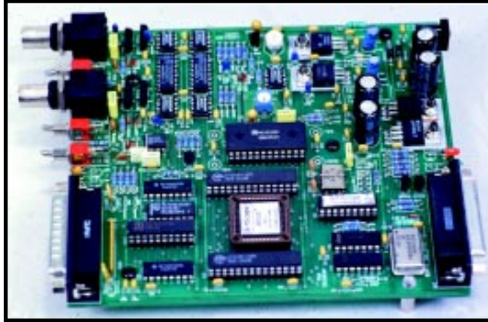
Photo 1 —BitScope was prototyped on a two-layer PCB. Notice that the components are arranged to separate analog and digital sections of the circuit.
