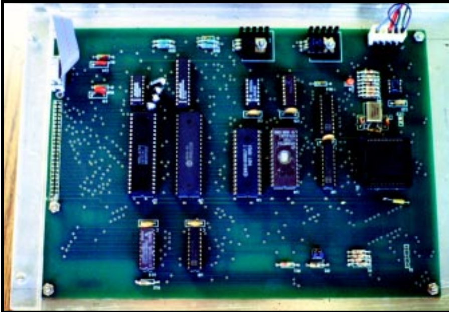
Photo 2 —The clear plastic strip to the left on the programmer's main circuit board is a hold down to prevent excessive flexing of the board when programming modules are installed.
