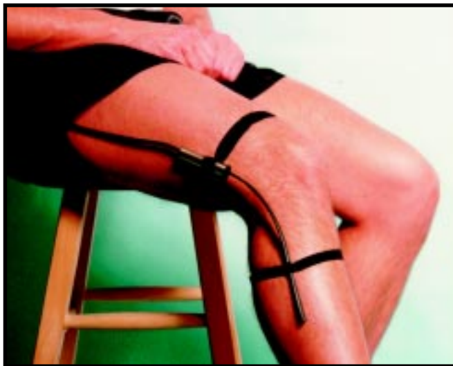
Photo 3 —Measurand Shape Sensors put a unique twist on position detection by translating curvature to force, acceleration, velocity, and flow.
