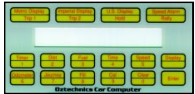
Photo 1—A specially manufactured color membrane keypad gives the car computer a professional look and feel.
