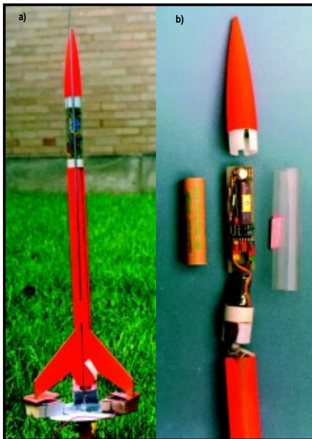
Photo 1a —Here's our smart rocket on the launch pad. Note the clear payload compartment containing the data-acquisition system and the copper contacts beneath the fins. The brown streak down the right side of the rocket is one of the two lines of conductive paint that bring the trigger signal to the payload. b —In this view of the data-acquisition system, you see the modifications made to the payload compartment. The brown patch on the rear bulkhead connector is conductive paint that forms a sliding electrical connection with the rocket body. To the left of the circuit board is a model-rocket engine.
