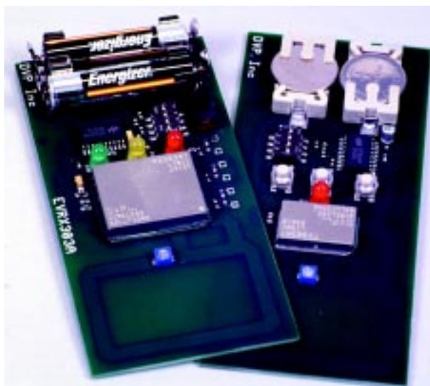
Photo 3— The batteries are included, and there are even blinking lights for me! Don't overlook the loop antenna etched onto the board.
