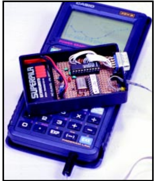
Photo 1 —The circuit fits inside a small plastic box just as large as the calculator. The micro jack connector hangs out, connecting to the calculator serial port. The box is stuck to the bottom of the calculator for operating. This arrangement gives the calculator a stable and comfortable slope.
