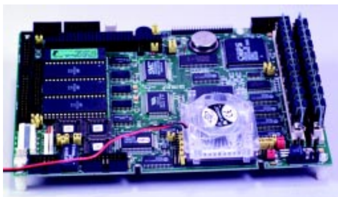
Photo 1—The SSD is contained in the three 29C040s right above the BIOS EPROM.
