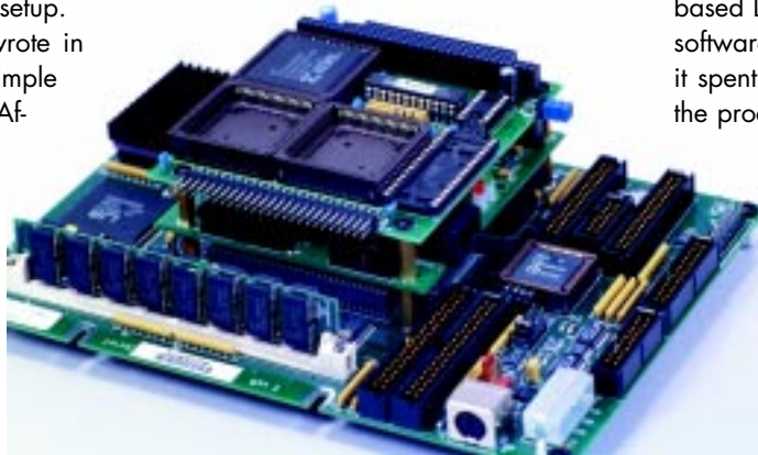
Photo 1—Our demo system consists of a CPU module on the bottom and an NE2000 Ethernet card module and a PF2000 module on top.
