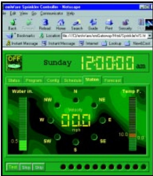
Photo 1 —The GUI can match the device interface or add to the functionality available on the device. This weather-station interface provides an easy, intuitive view of weather conditions, enabling the user to see the impact of changing data on the device functions.
