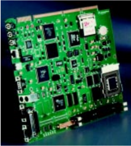
Photo 1 —The Motorola NLX55 motherboard features a Pentium MMX CPU, graphics controller, and 10-/100-Mbps Ethernet controller. Unique to this board, it also includes a socket for a SanDisk flash-based ATA card.
