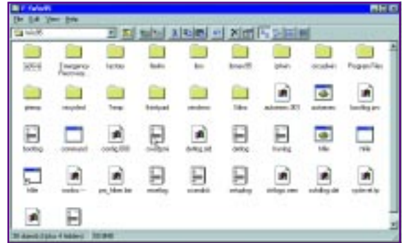
Photo 3 —Here's a screenshot of the Windows NT machine in my basement office mapping my hard disk on my notebook. The notebook has a wireless LAN card and is currently on the kitchen table. Linux also enables me to mount my Windows 95 partition on my notebook and make it available over the network. So now I can map a Linux-based volume, which has a Windows 95 partition mounted on it, all from Windows NT over a wireless LAN.
