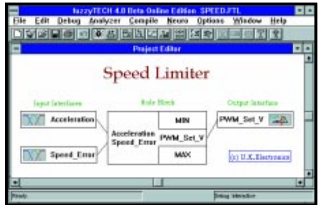
Photo 1—The fuzzy-logic controller for the speed limiter uses acceleration and speed error as inputs to determine the set value for the pressure valve.
