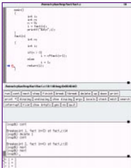
Photo 1—The X Windows version of the GNU debugger (xxgdb) has a source window, a command-line window, and an extra window to display variables. These are features you'd expect from a source-level debugger.
