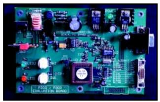
**Photo 1**—The Intellon P300 evaluation board shows the proper implementation of the power-line communication ICs in an easy-to-probe package.
