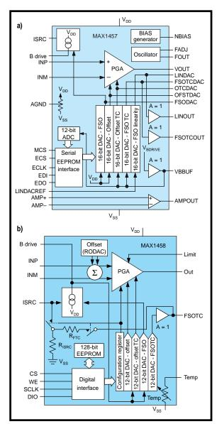
**Figure 2**—Earlier Maxim parts, the MAX1457 (a) and MAX1458 (b), targeted the same bridge sensor applications but required support from an external ADC and micro.
