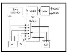
Figure 1—In this diagram of the video switch, the signals flow from left to right. The DAC outputs can provide a regenerated sync signal or some other video test pattern.
