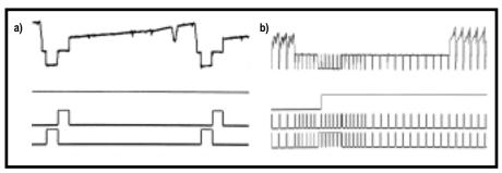
Figure 6—The top lines show the video input signal, and the second lines show the field output of the PLD. The third lines show the color burst active signal, and the bottom lines show the horizontal sync signal. **a**—Here you see a complete scan line and the horizontal sync on either end of it. **b**—Here are many scan lines containing a vertical sync.
