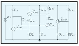
Figure 1—Here's the full schematic of the Schmitt-trigger sensor which features high input impedance and full output swing along with less current burden on the thermistor.
