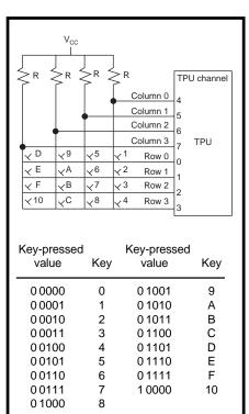
**Figure 4**—Here's the hardware setup for 4 × 4 matrix keypad decoding. As you see, it requires eight TPU channels—four input channels for the rows and four output channels for the columns.
