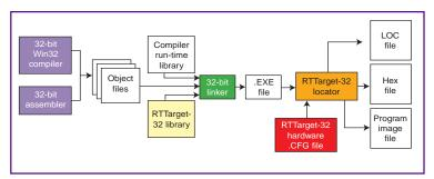
Figure 3—This diagram illustrates creating a binary program image file with standard Win32 compilers and the On Time Embedded RTOS.
