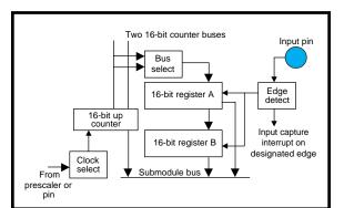
Figure 2—Here's a MIOS double-action submodule configured for input period measurement mode. There are two 16-bit buses between the 16-bit up counter and data registers A and B.
