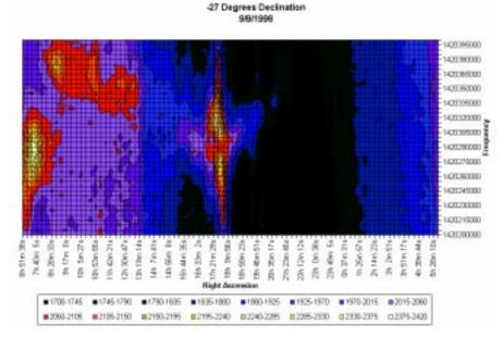
Photo 2—This radio map of the sky was created by Daniel Boyd Fox (a local amateur astronomer) with a 16-foot dish antenna and an ICOM R7000 communication receiver. He wrote a program (SETIFOX) to calculate the spectral data. The emission in the middle (around RA 18h) is caused by our galactic center, and the dentrils above and below are the spectra of the Doppler-shifted hydrogen emission of stuff moving away (lower frequency) and approaching (higher frequency).
