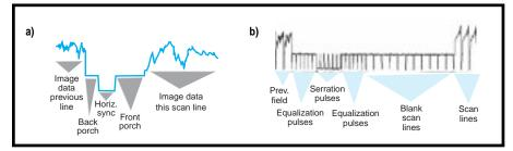
**Figure 3a**—This figure depicts a horizontal sync signal between two scan lines. Time advances along the horizontal axis and the voltage is shown on the vertical axis. **b**—This figure depicts a vertical sync between two fields. Voltage is on the vertical axis and time advances along the horizontal axis.
