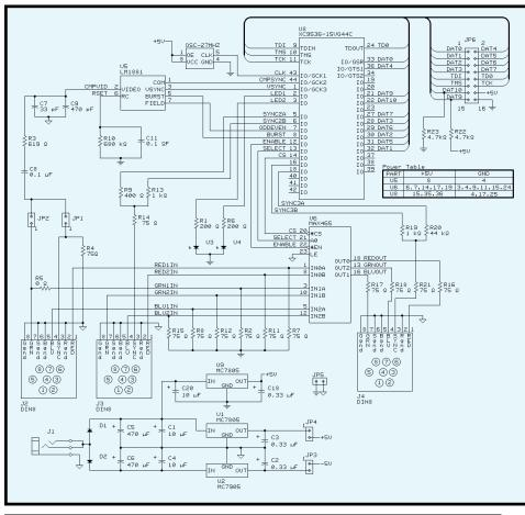
**Figure 4**—In this schematic, signals generally flow left to right. The +5 V off of JP4 drives only the analog chips, whereas the other +5 V drives all of the digital chips.
