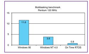
Figure 1—The benchmark performs 400,000 semaphore operations with 200,000 task switches. The times shown here are for a 120-MHz Pentium.
