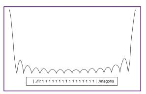
Figure 2—This graph shows the spectral response of a 16:1 decimation filter. The filter is crude but can be implemented efficiently. A sharper filter can be implemented at a lower sampling rate if necessary.
