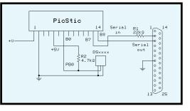
Figure 3—Here, I used a PicStic as a 1-wire interface controller. Calls to assembly-language routines from BASIC enable me to quickly write simple applications using 1-wire sensors. Output messages go to either a PC or a serial LCD.
