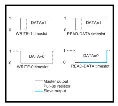
Figure 1—After an initial low output, both write and read timeslots can hold the output low indicating a data bit of 0. When writing, the master controls the data, and when reading, the slave controls the data.
