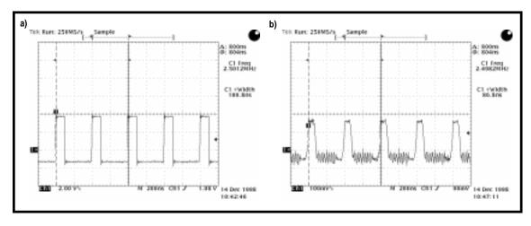
Photo 1a—The scope capture of the MPC555 MIOS PWM output shows a 2.5-MHz 25% duty cycle signal with a fast slew rate. The pulse width is measured at 100 ns or 25% of the 400-ns period. b—This scope capture of the MPC555 MIOS PWM output shows a 2.5-MHz 25% duty cycle signal with a slow slew rate. Note the volts per division scale compared to Photo 1a.
