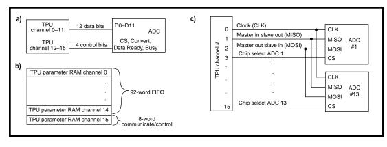
Figure 6—Diagrams (a) and (c) show how the TPU can be used to control ADCs and store the data in TPU parameter RAM, which acts as a FIFO (b).
