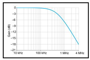
**Figure 5**—The calculated filter response has a nearly –18-dB effect on the color burst signal and little effect on the sync signal, which is mostly under 500 kHz.
