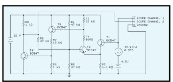
Figure 2—The output response of the sensor was checked on Electronics Workbench. Here, the thermistor RT is replaced by a sine-wave generator to facilitate simulation.
