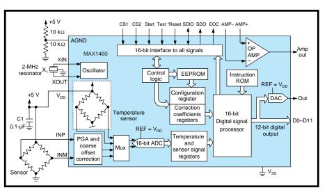
**Figure 1**—The MAX1460 combines everything needed to accommodate a variety of bridge-type sensors. Major integrated functions include a programmable gain amp (PGA), 16-bit ADC, temp sensor, and 16-bit processor.
