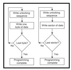
**Figure 1**—A tale of two programming models: the lefthand side (Am29F040B) requires an unlocking sequence after every byte is programmed, and the right-hand side (AT29C040A) requires an entire sector of memory to be programmed each time you write to the flash.
