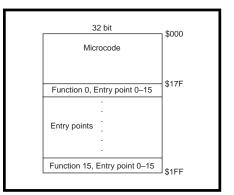
Figure 3—In the '68332, the 2 KB of onboard RAM is divided into 1 KB for microcode and 1 KB for program entry points. The microcode instructions are 32 bits long. The formatting details were covered in Part 3.
