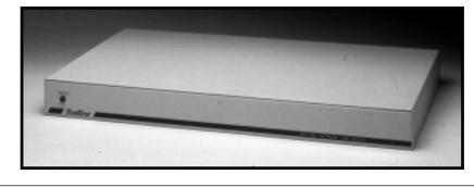
The NTS-90 is also a source for accurate serial time broadcasts and time on demand. A once-per-second time broadcast (accurate to the millisecond) is available via the serial port. The NTS-90 can also timestamp external events with millisecond accuracy.
