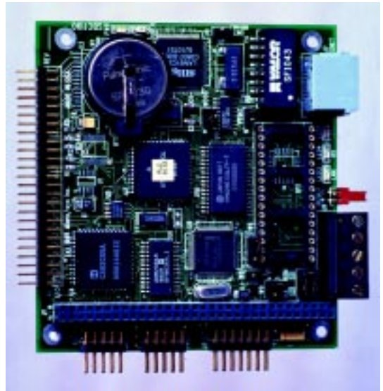
Photo 1—The Ethernet circuitry is between the battery and the Ethernet connector. ADC and DAC capability can also be added under and around the battery.
