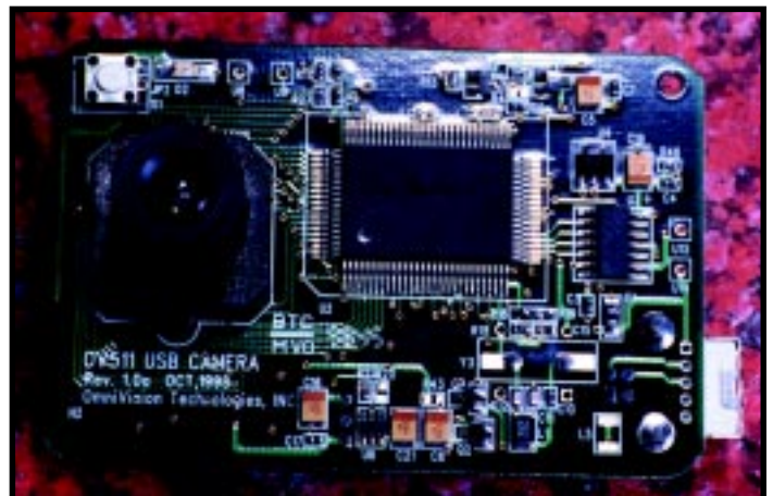
Photo 1—USB is finally on the move (ironically, thanks to blessing by the iMacs), and OmniVision follows suit with a highly integrated USB camera design.
