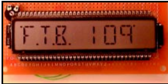
Photo 1 —Two I 2 C PCF8566 LCD segment drivers can drive all 144 segments on this eight-character display. The driver ICs can be seen behind the LCD's glass.
