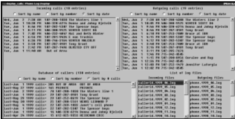
Photo 3—The display_callers function shows incoming calls, outgoing calls, a list of all past callers, and a pick list of the logs for each month.
