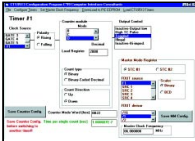
Photo 2—Configuring each timer section is accomplished from the main screen of the Visual Basic host program.
