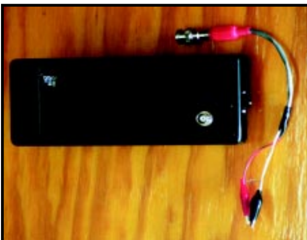
Photo 2 —There are no knobs or switches on the Count-4. Just plug in the power supply and hook up the input.
