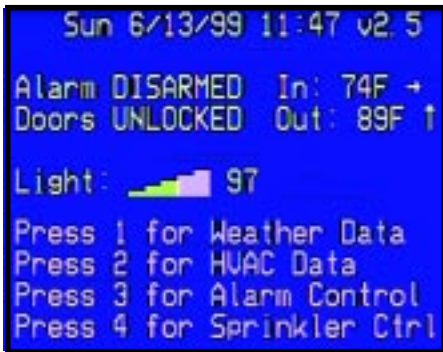
Photo 2 —The PIC-TV can generate detailed color backgrounds at the screen, grid, or character cell level. This allows it to draw attention to urgent information.
