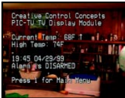
Photo 3 —The BOB-II can generate its own backgrounds if no external video signal is used. All text is monochrome when overlaid on an existing video signal. An ideal application of this mode is to use a security camera image as a background.
