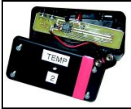
Photo 1 — Here is the inside of a transmitter module. On the circuit board are PIC that does the Poisson calculations, and the pushbuttons and LED that make up the (minimal) user interface.
