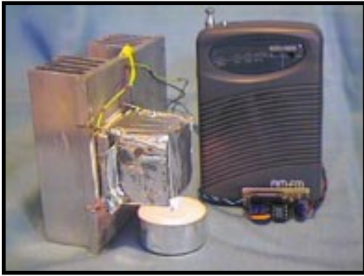
Photo 1 — The candle-powered radio shown here uses a reverse-mode thermoelectric cooler to convert heat into electrical energy. Power is boosted to a usable level by a step-up switching regulator, which powers the AM/FM radio.
