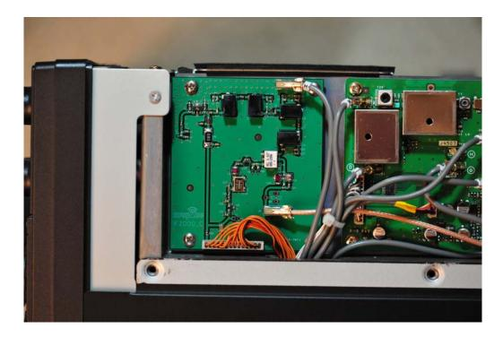
7. Insert small Taiko Denki connector and cable end though back of FT-2000 as shown. If the small coax connector does not fit, it is OK to compress the sides of the connector slightly using a pair of pliers.
