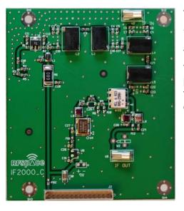
The IF-2000 Revision-C IF interface board adds an IF output at 10.55 MHz to the Yaesu model FT-2000 and FT-950 transceivers. This board allows the interfacing of the transceiver to an RFSPACE SDR or panoramic adapter. The addition of an SDR to the Yaesu radios greatly enhances its capabilities.
