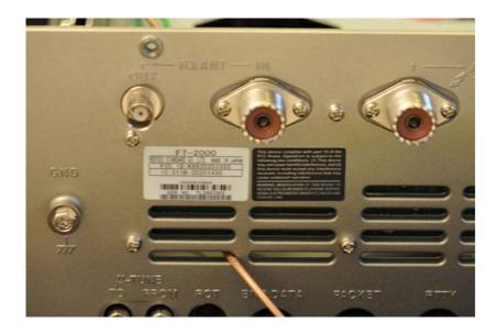
8. Route coax cable as shown and connect to IF OUT connector at position U6.
