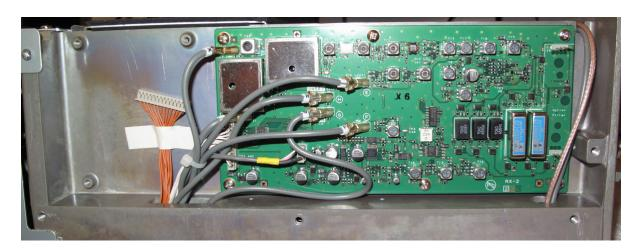
4. Install IF-2000 into DMU-2000 position as shown using the 4 screws supplied.
