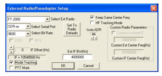
After adjusting the setting in SpectraVue as shown above, verify that the FT-2000 or FT-950 and SpectraVue are tracking. When the VFO on the radio is changed, the software should update the frequency and vice versa. If this does not happen, there is a communications problem. Check the serial cable and the radio menu settings 027 and 029.
